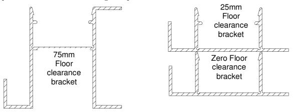
2 Two floor fixing brackets and two top brackets are supplied with each length of side flue ducting. A bracket should be positioned approximately 150mm (6") from the end of each length of duct. See Figure 19.
